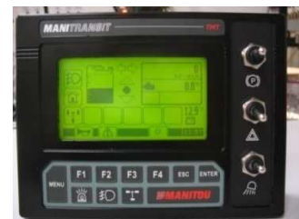
New digital instrument panel with reinforced electrical sealing
