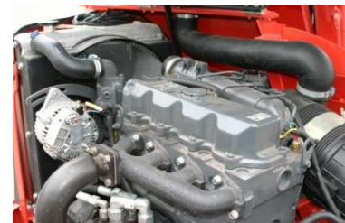
Kubota 50 HP Interim Tier 4 - Stage III A engine with improved cooling system and reduced polluting emissions
